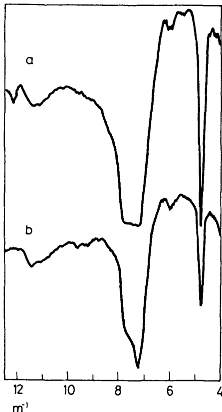
Fig. 3 Infrared spectra of \text{K}_2\text{SiF}_6 and \text{K}_3\text{SiF}_7
